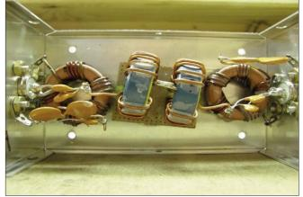
This is the 15-Meter BPF. The right side is the input (transceiver) side and the left is the output (antenna) side. The top set of capacitors on the right side tunes the input to 50 ohms. The lower set of capacitors tunes the input to output circuit. The lower
