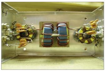
This is the 20-Meter BPF. The right side is the input (transceiver) side and the left is the output (antenna) side. The top set of capacitors on the right side tunes the input to 50 ohms. The lower set of capacitors tunes the input to output circuit. The lower set of capacitors on the left side tunes the output to 50 ohms. The top set of capacitors tunes the input to output circuit. This one took 13 capacitors to tune it up.
