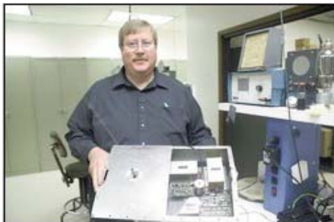
ARRL Lab Test Engineer Bob Allison WB1GGM, holds a newly functional OSCAR I. The satellite is shown with its cover open to the left, making the bird appear twice as large as it actually is.
