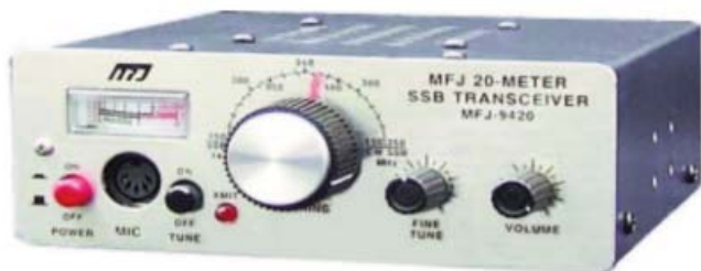
This radio tunes the 20 meter amateur "voice" band (14.150 Mhz to 14.350 Mhz.).
