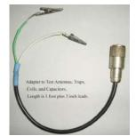
Use the type of RG58 that has a stranded center conductor. The overall length is approximately 1 foot but not critical. Suggest about 3 inch leads.
