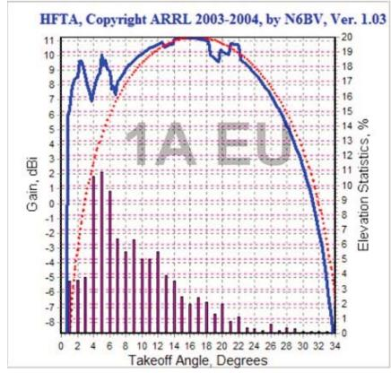
HFTA Terrain analysis comparing vertical radiation angle towards Europe including terrain effects at one site with same antenna over ideal flat ground.
