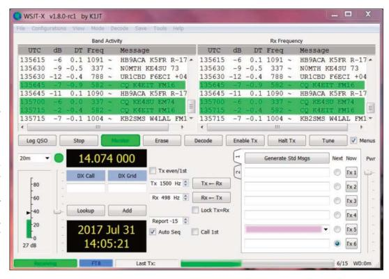
The new mode is named after its developers, Steven Franke, K9AN, and Joe Taylor, K1JT. The numeral designates the mode's 8-frequency shift keying format. Tones are spaced at 6.25 Hz, and an FT8 signal occupies just 50 Hz. Unlike JT65 or JT9, transmit and receive cycles in FT8 each last about 15 seconds. Like JT65, FT8 requires accurate time synchronization. An auto-sequencing feature offers the option to respond automatically to the first decoded reply to your CQ.
