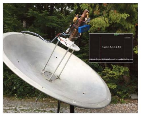
In a Software Defined Radio, computers digitally perform the signal mixing and amplification functions of circuits that used to be analog; software has replaced hardware. SDRs are cheap, sensitive, and they give hams the kind of exquisite control over frequency required to tune into distant spacecraft.
