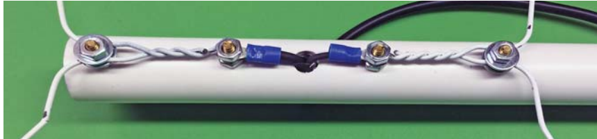
Figure 4 — Closeup of the feed point and hanger mounting.
