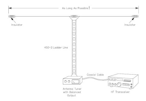
• Figure 1 Cut a long length of multistranded copper wire into two equal pieces. Attach the pieces to each end of a plastic or ceramic insulator and place two more insulators at the two ends. Attach 450-O ladder line at the center and run it back to your antenna tuner. Secure ropes to both ends and raise the antenna as high as you can. You now have a dipole antenna that you can use on several HF bands.
